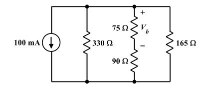
Use the nodal analysis method to determine the value of  $V_b$ .
